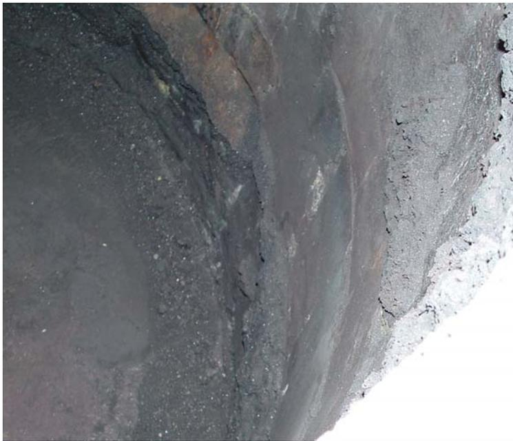
**Figure 8: Viewed from the top it is clear that no significant wear of the lining has occurred.**
