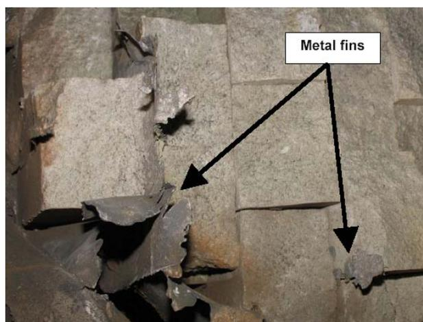
**Figure 2: Iron penetration into the hearth found after a refractory break-out on a DC-ilmenite smelter [3]**
