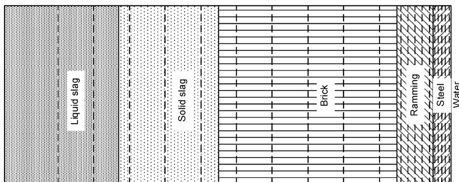
Fig. 2. Schematic representation of the structure of the Wall Model.
