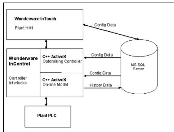
Figure 4 – Layout of implemented advanced process control system.
