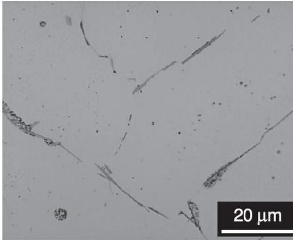
Figure 1 - Example microstructure before homogenising<sup>3</sup>.
